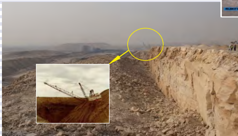
Blast carried out at Reliance Power, Sasan coal block using more than 300 tons of customised explosives for dragline equipment ( inset ). Images are taken by high speed cameras of the Technical Services Group along with the Blasting Team
