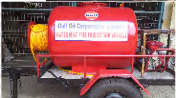
In-house developed mist spray machine ( inset ) The machine was inspected by government authorities tested and approved for fire fighting
